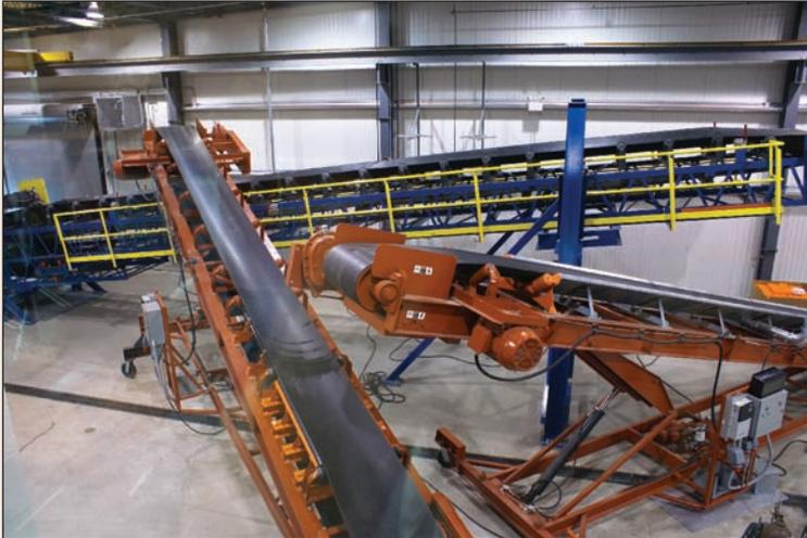
At the Center for Innovation, the process simulation area incorporates a three-belt recirculating conveyor loop carrying materials for observation of material flow and component life.
